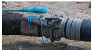
Non Sphere Lock<sup>™</sup> handles tied down with rope, susceptable to unwanted opening.
